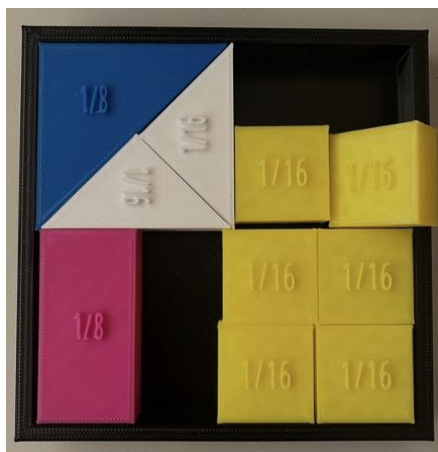
Figure 20. Mismatch between printed box and manipulative dimensions (group 1).
