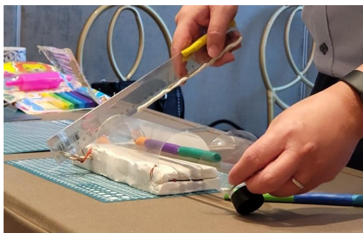
Figure 8. Group 7 prototype that was like Group 4 and 5 prototypes. However, the vegetables would not be attached to the pusher.
