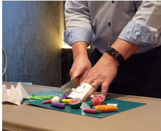
Figure 3. Group 2 prototypes comprise the folded paper (left) and plastic shield with a horizontal ice-cream stick for distancing the knife.
