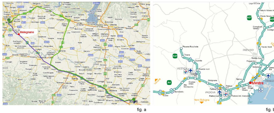
FIGURE 6. fig. a The shortest road from Milano to Bologna pass through Melegnano (blue road). If Melegnano is blocked, the shortest road is the one passing through Brescia (green road). This behaviour is exactly predicted by the interference analysis. fig. b . Mestre is a critical node to connect Trieste with the rest of Italy. Notice the recently built alternative path passing through Spinea, called “passante of Mestre”.
