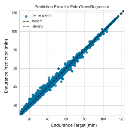
Figure 10. ET surrogate model predicted endurance values compared to the target physics-model estimated values.
