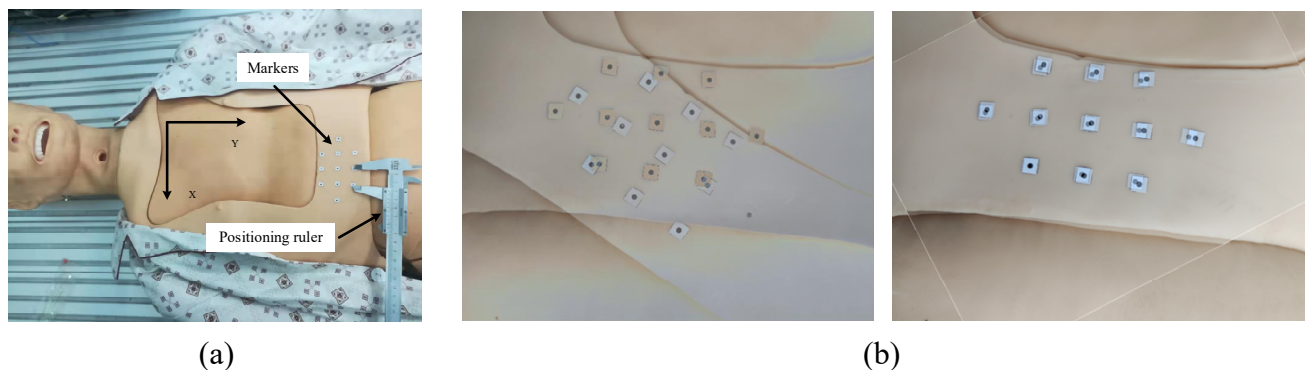
Figure 15. (a) The markers are pasted on the surface of the mannequin, and (b) comparison diagram before and after three-dimensional registration based on improved algorithm.
