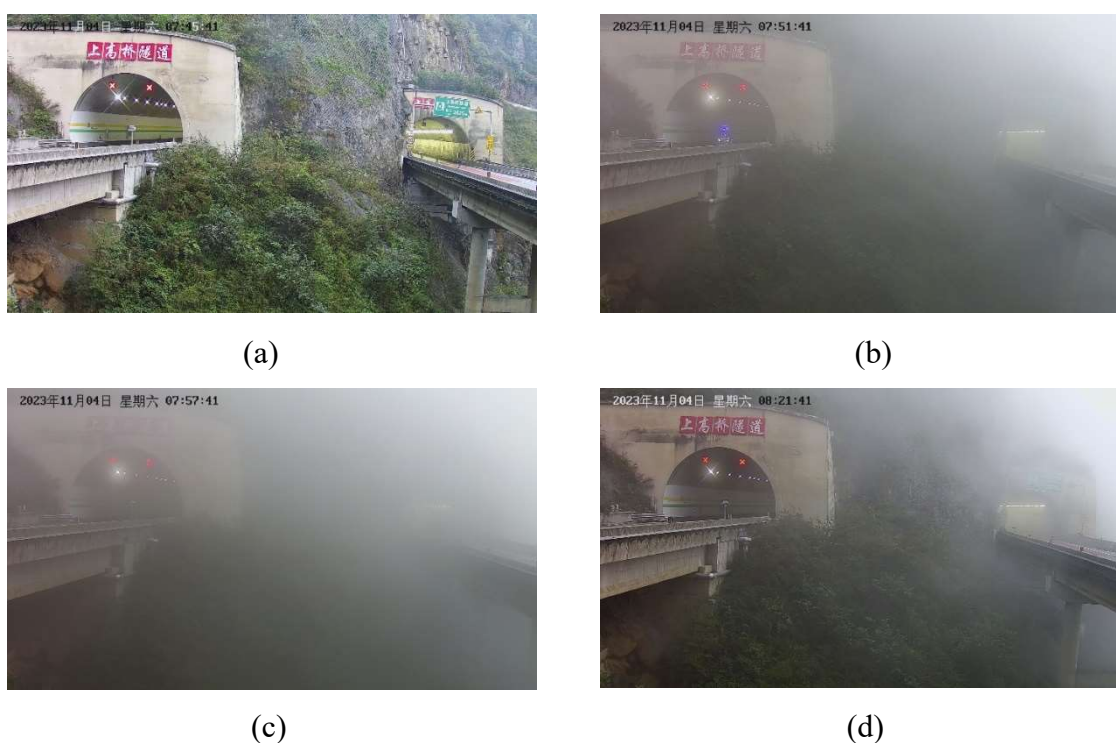
Figure 1. Actual scenes of highway visibility changes. (a) visibility 8880 m (datetime: 2023-11-04 07:45:41). (b) visibility 837 m (datetime: 2023-11-04 07:51:41). (c) visibility 105 m (datetime: 2023-11-04 07:57:41). (d) visibility 1157 m (datetime: 2023-11-04 08:21:41).
