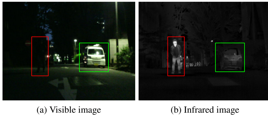
Figure 3. Illustrations of registered infrared and visible images, where infrared and visible images have unique (the red box) and common (the green box) information.
