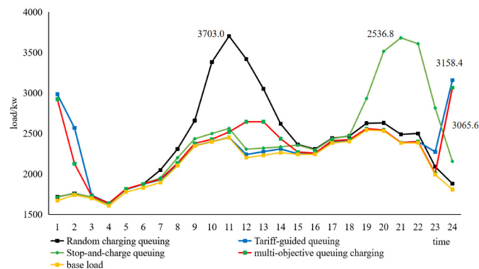
Figure 12. Base load with 1000 vehicles charging load superimposed under different strategies.
