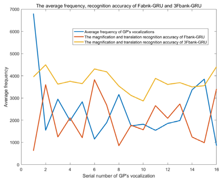
Figure 9. The average frequency of GP's vocalizations (the blue curve), the magnification and translation versions of recognition accuracy using Fbank-GRU (the red curve) and using 3Fbank-GRU (the orange curve). In order to observe the change trends of recognition accuracy using Fbank-GRU and 3Fbank-GRU and the relation between each of model and the average frequency of GP's vocalizations, the recognition accuracy of two models was magnified by 40,000 times and subtracted by 35,000 to let them be of the same order of magnitude as the average frequency. The x axis shows the serial number of GP's vocalizations defined in Table 1.
