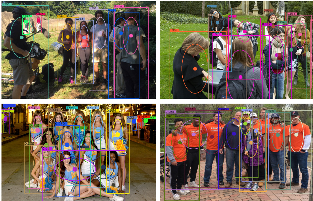
Figure 8. Distribution of attention points decoupled by our proposed DMCA to predict the class confidence. Each ellipse's long and short axes are the horizontal and vertical distributions' standard deviation of the attention point set, and each ellipse's center is the weighted average of the attention points.
