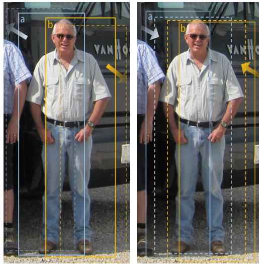
Figure 1. The synchronous update of the prediction boxes in the fine-tuning stage. The solid boxes a and b represent the prediction boxes in the current fine-tuning stage by the decoder blocks, and the dashed boxes represent the possible synchronous updates after fine-tuning by the symmetric decoder structure.
