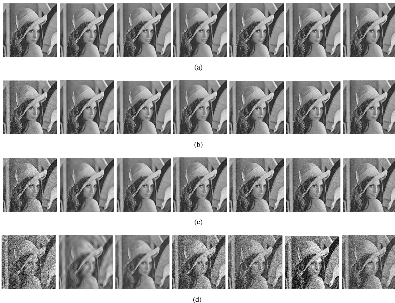
Figure 17. Denoising results of the Lena image for different values of noise level (see column 1 located on the left side of the figure). The algorithm used, Shearlet method, TV method, Bilateral Filtering, Trilateral Filtering, and Compressed sensing are arranged in columns 2, 3, 4, 5, 6 and 7, respectively.
