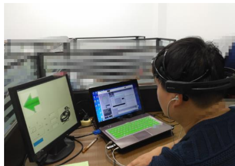
Figure 3. Schematic diagram of wearing 16-lead Emotiv EPOC+ helmet instrument.
