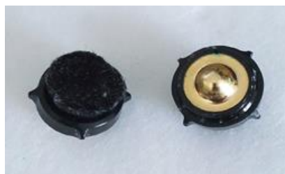
Figure 2. Wet electrode of helmet instrument.
