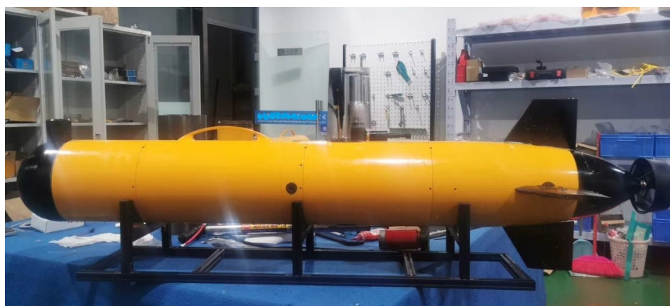
Figure 1. The AUV for hardware assembly and system debugging in the laboratory.
