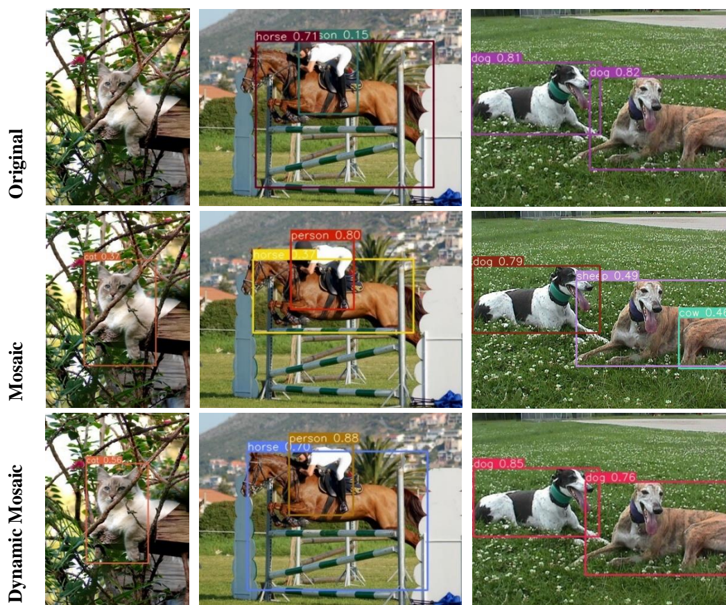
Figure 8. Comparison of detection examples of different data augmentation schemes. The detection example comes from the test set of Pascal VOC 2007. It can be seen from the detection results that the detection model using the Dynamic Mosaic algorithm can recognize the target object more accurately, and there is no missed detection or false detection.
