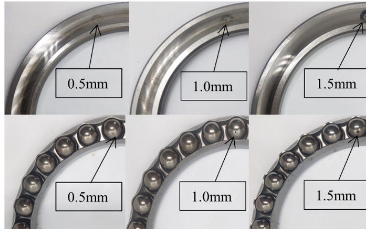
Figure 6. Partially enlarged view of bearing component failure.
