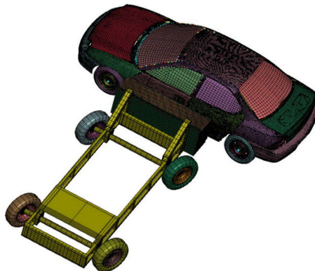
Figure 12. Three-dimensional model diagram of the car side crash [54].
