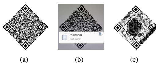
Figure 13. Rotation test results: (a–c) shared QR code, decoding information and secret recovery at 45^\circ rotation.
