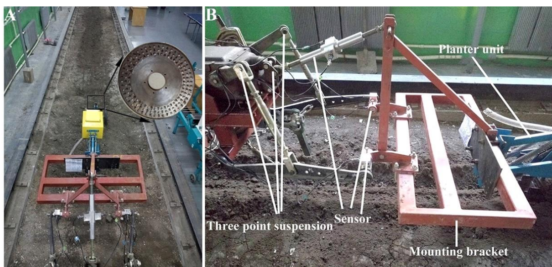
Figure 3. (A) Soil bin and (B) experimental device.
