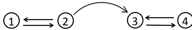
Figure 4. Two blocks that are non-strongly connected. The 1st and 2nd compartments (involved in block-1) are strongly connected and also for the 3rd and 4th compartments (involved in block-2), but the only connection between the two blocks is from the 2nd compartment to the 3rd compartment.
