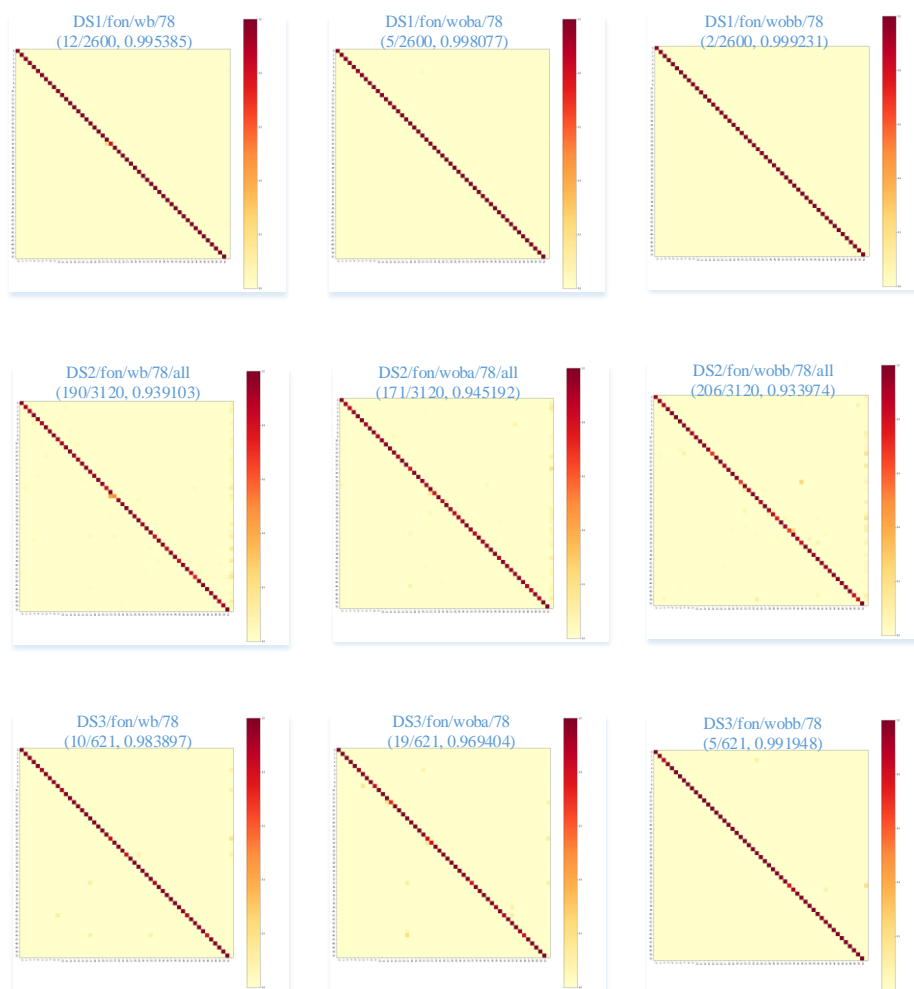
Figure 6. Confusion matrices of the signage object detection results (with image flip-On setting). The rows from top to bottom are for dataSet1 (DS1), dataSet2 (DS2), and dataSet3 (DS3) respectively; the columns from left to right are for the three bounding boxes: with-boundary (WB), without-boundary type-A (WoB-A), and without-boundary type-B (WoB-B).
