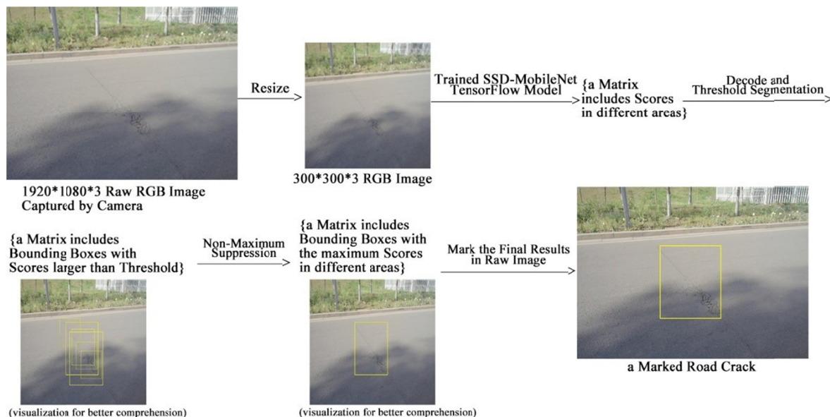
Figure 6. Process of detection on an example image.
