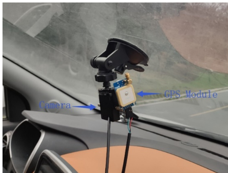
Figure 3. Usage example of our system. A camera and a GPS module hang on windshield of a car.
