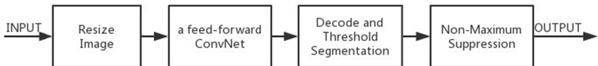
Figure 5. Core process of the detection algorithm [5,6].
