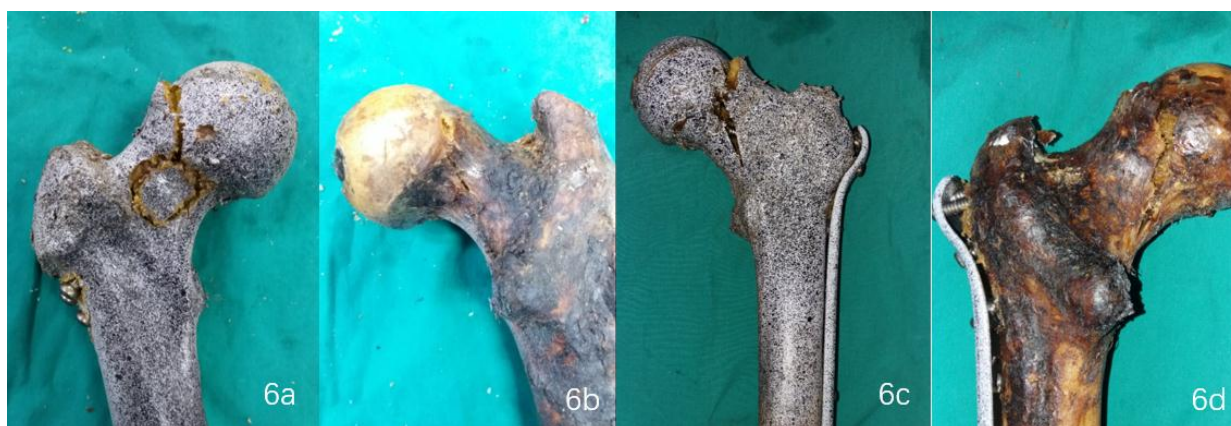
Figure 6. The fracture lines of the axial loading failure of group 1 ADH on stage 3 (a,b) and group 1 LDH on stage 3 (c,d) were similar, which began from the super-lateral region between the femoral head and neck, then went down straightly, and stopped above the lesser trochanter, with the lesser trochanter not involved.
