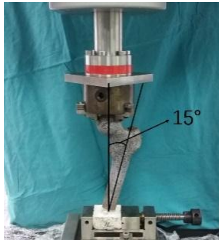
Figure 2. The angle between loading axis and the proximal shaft was 15^\circ during the mechanical testing, which was in a one-legged stance.
