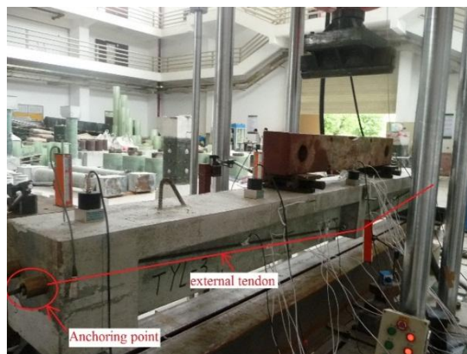
Figure 4. Profile of the external tendon.
