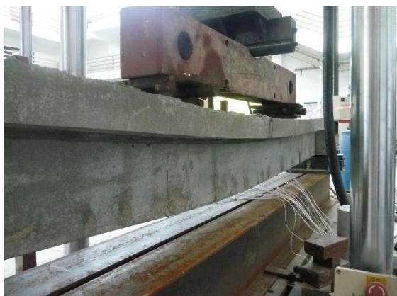
Figure 8. Failure mode of S-0 beam.
