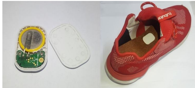
Figure 4. The wireless data acquisition unit embedded a 3-axis accelerometer and the placement in a sneaker.
