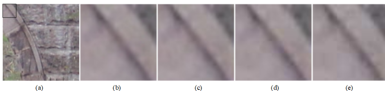
Figure 3. JPEG compression visually disturbs resampling trails. (a) Upscaling 150% uncompressed; (b) Magnified boxed local region in (a); (c)(d)(e) JPEG compressed versions of (b) with Q = 90, 70 and 50 , respectively.
