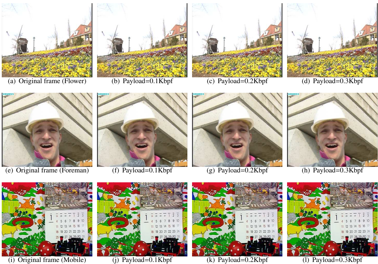
Figure 7. Visual quality of original and stego frames for Flower (frame 48), Foreman (frame 30) and Mobile (frame 63). The relative payloads are 0.1 Kbpf, 0.2 Kbpf, and 0.3 Kbpf.
