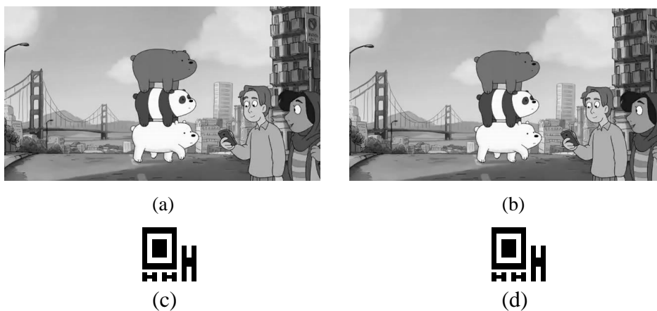
Figure 7. (a) original video, (b) watermarked video, (c) original watermark, (d) extracted watermark.
