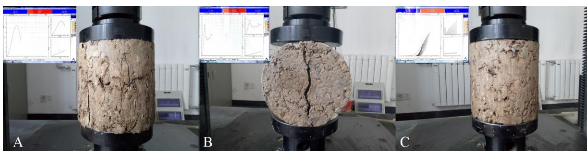
Figure 3. Mechanical property tests: a: unconfined compressive strength test; b: splitting strength test; c: compression rebound modulus test.
