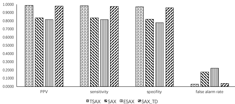
Figure 5. The comparison of four metrics with four methods, the above three are the higher value the better, and the false alarm rate is the lower value the better. The first column is TSAX.
