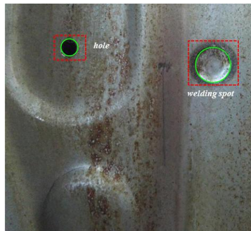
Figure 11. Wrong detection result example. The hole in the BIW was mistakenly identified as a welding spot.
