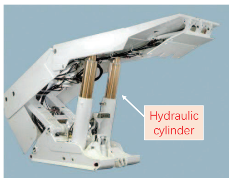
Figure 3. Structure of the hydraulic support pushing mechanism.
