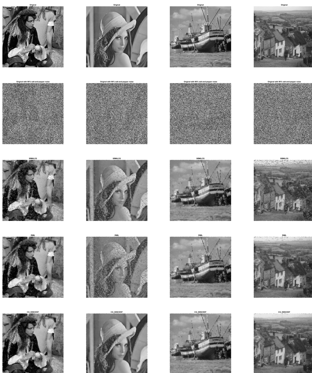
Figure 6. The original image (1st row) with (2nd row) 90% salt-and-pepper noise, the restored images by SRMLCG(3rd row), RMIL (4th row), and CG_DESCENT (5th row).
