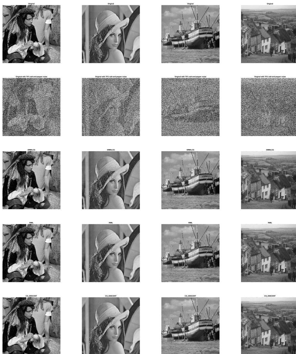
Figure 5. The original image (1st row) with (2nd row) 70% salt-and-pepper noise, the restored images by SRMLCG(3rd row), RMIL (4th row),and CG_DESCENT (5th row).
