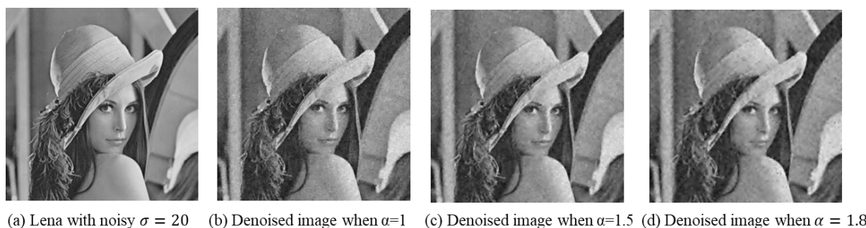
Figure 3. Comparison of visual results with different values of \alpha for the noisy image at \sigma = 20 .
