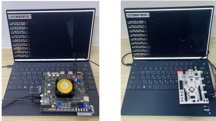
Figure 10. Execution of the prototyped QC emulator on the Kintex Ultrascale+ FPGA board (left), and on Arty A7 FPGA board (right).
