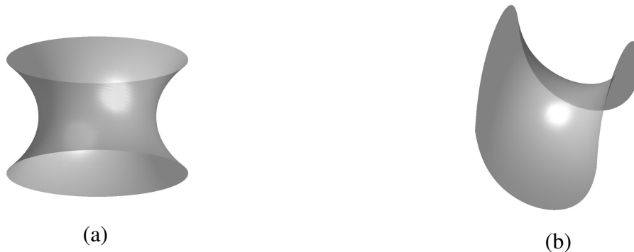
Figure 2. (a) Catenoid, and (b) Scherk's first surface. Two surfaces are generated by the analytic formulations, derived by the Weierstrass-Enneper representation.
