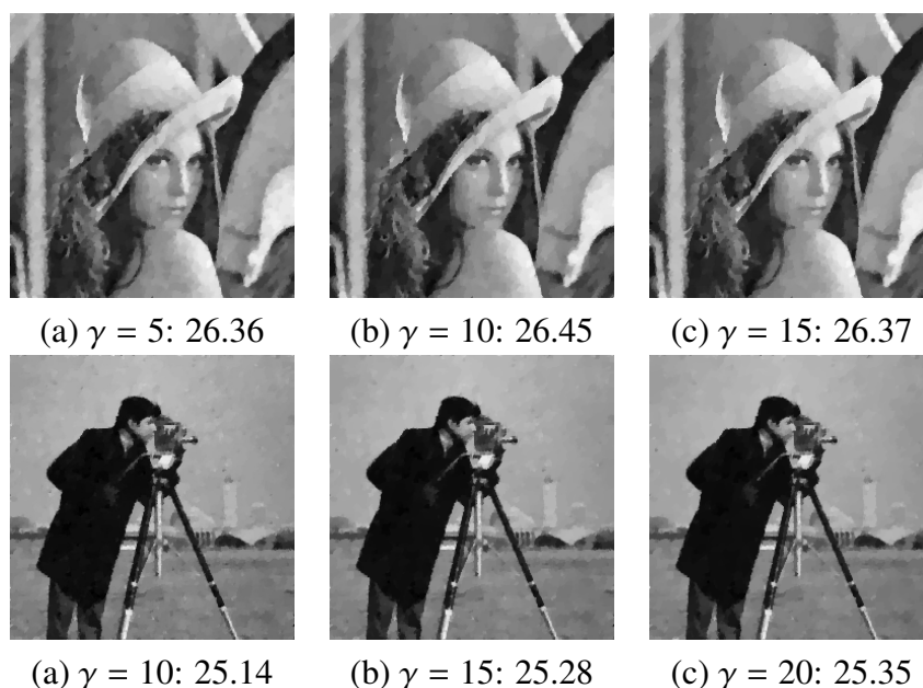
Figure 17. Denoising results with different \gamma in the proposed model, when (\gamma_*, \sigma) = (10, 20) (top row), (\gamma_*, \sigma) = (15, 10) (bottom row). PSNR values are presented. Parameter \lambda_2 (left to right): (top) 9, 20, 31, (bottom) 22, 30, 38.
