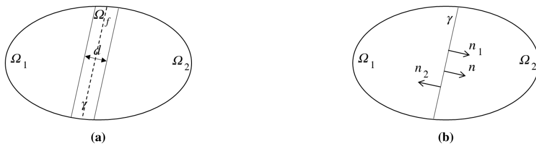
Figure 1. The hybrid-dimensional fracture model with one single fracture in two-dimensional domain. (a) Domain divided into two sub-domains \Omega_1 and \Omega_2 by a thin region \Omega_f . (b) Fracture \gamma modeled as one-dimensional domain.
