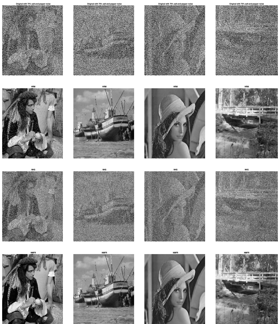
Figure 9. The noisy images with 70% salt-and-pepper (first row) and the restored images by HRM (second row), NHS (third row), and NMFR (last row).
