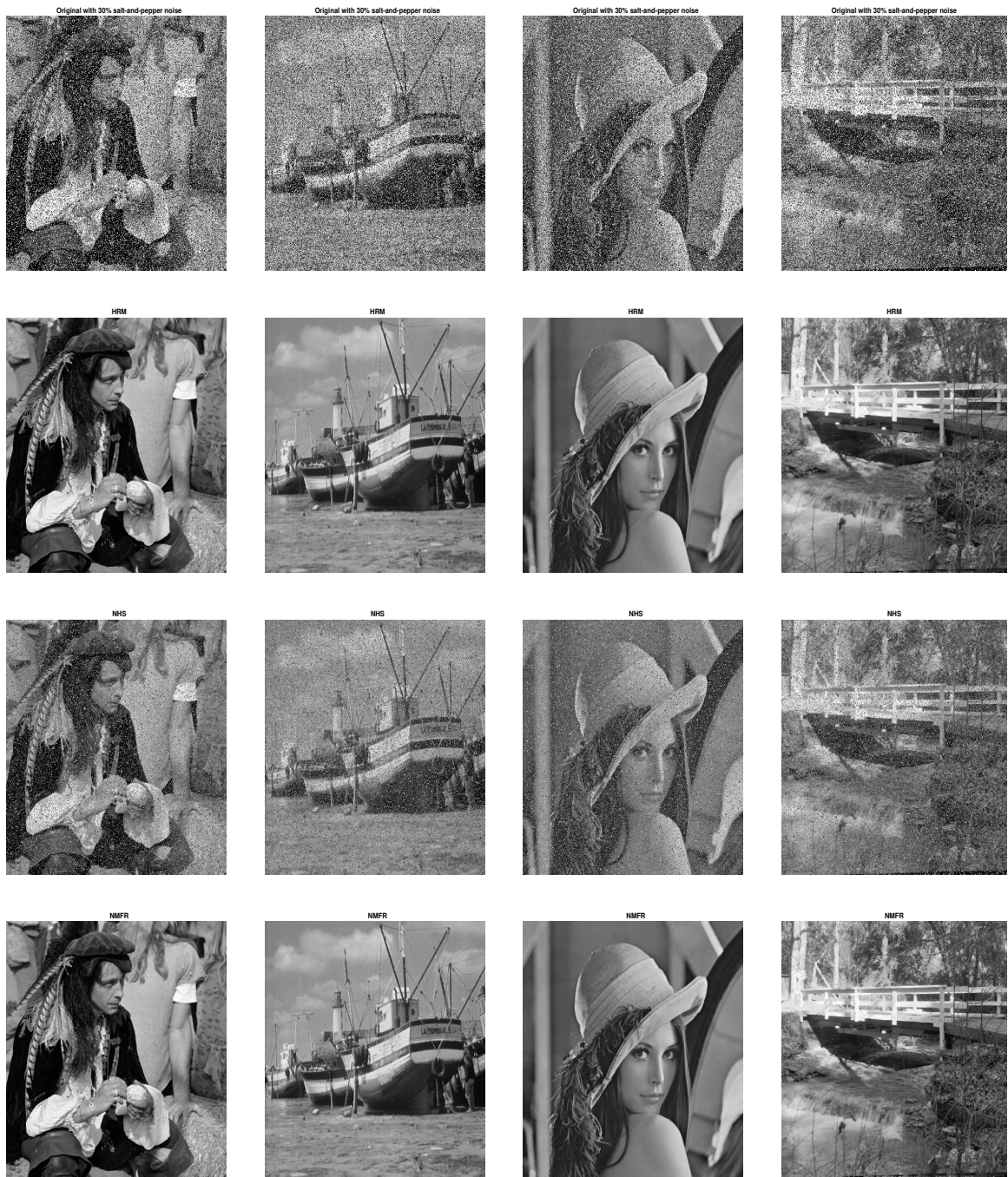
Figure 5. The noisy images with 30% salt-and-pepper (first row) and the restored images by HRM (second row), NHS (third row), and NMFR (last row).
