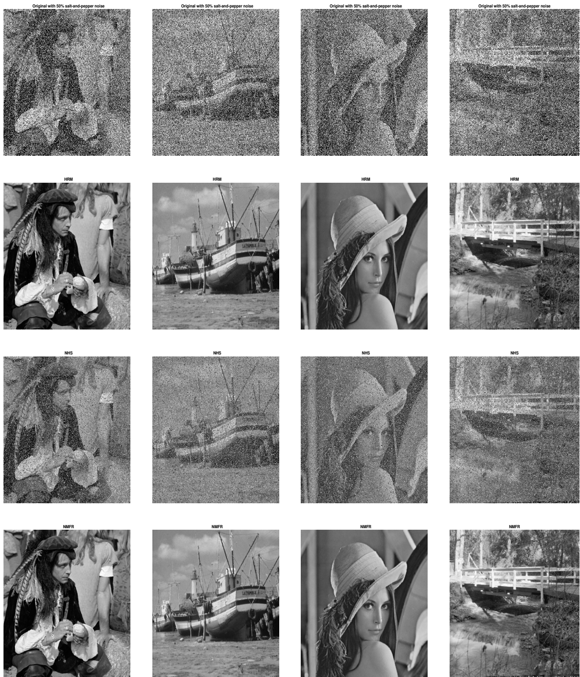
Figure 7. The noisy images with 50% salt-and-pepper (first row) and the restored images by HRM (second row), NHS (third row), and NMFR (last row).
