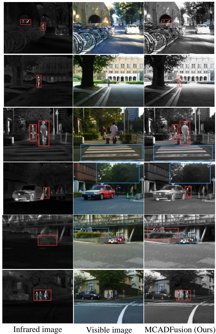
Figure 8. The images are sourced from the MSRS dataset. The left column displays infrared images, the middle column shows visible light images, and the right column presents the fusion results of MCADFusion applied to the MSRS dataset.
