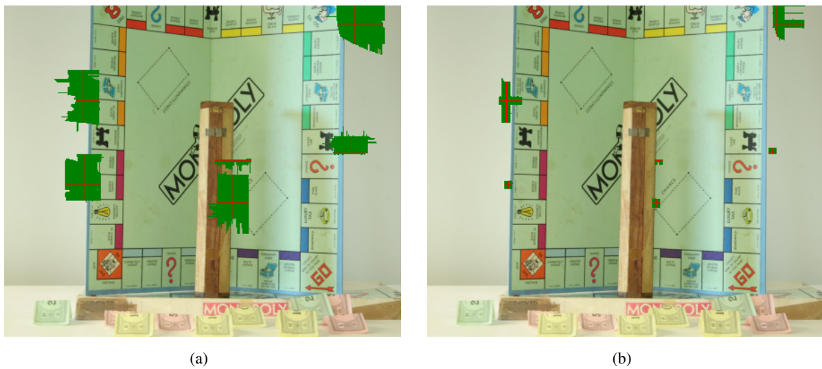
Figure 6. Examples of support windows on the Monopoly image. (a) Adaptive window based on the cross proposed by Mei et al. [13]. (b) Improved cross adaptive window.
