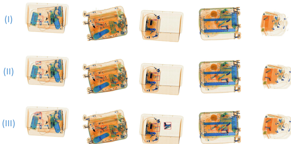
Figure 14. Samples of the synthesized X-ray inspection images in the pseudo-color mode. Each image comprises (I) one prohibited item (II), two prohibited items, or (III) two or more overlapping prohibited items.
