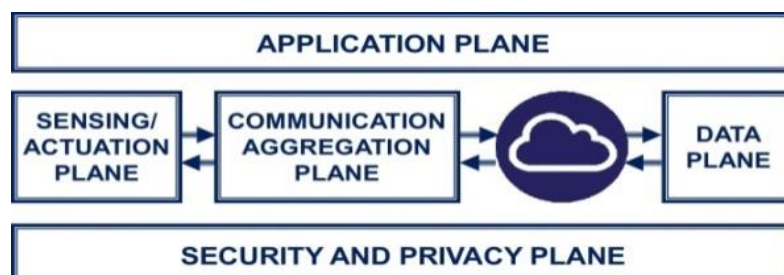
Figure 2. A high-level illustration of the architecture of smart city applications [16].
