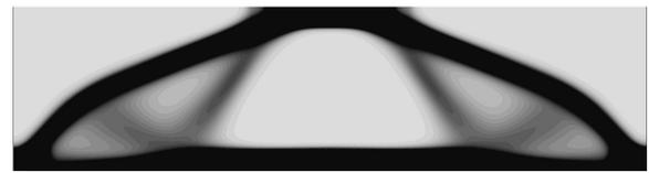
b1. The 50th iteration of homogenization structure.
