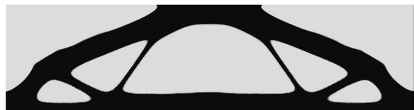
b4. The 300th iteration of homogenization structure.
