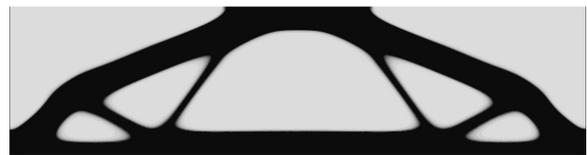
b2. The 100th iteration of homogenization structure.
