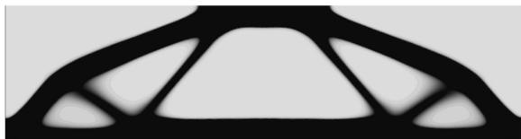
a2. The 100th iteration of composite material.
