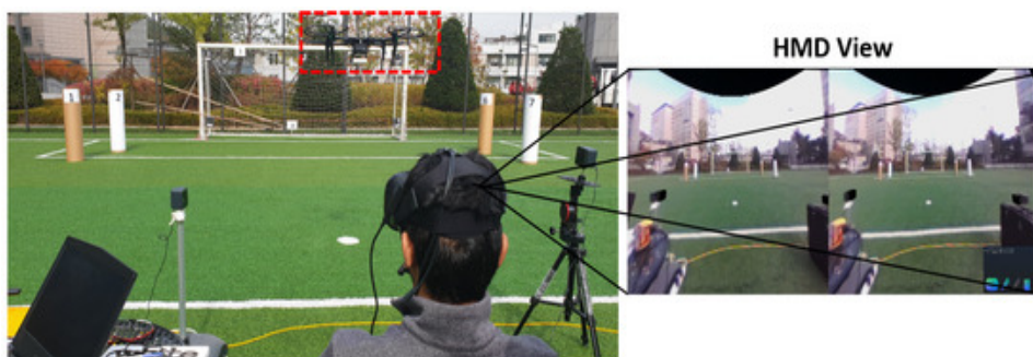
Figure 18. An eye-gaze-guided active immersive UAV (unmanned aerial vehicle) camera [112].
