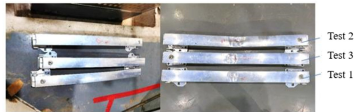
Figure 17. Bumper crash deformation analysis.
