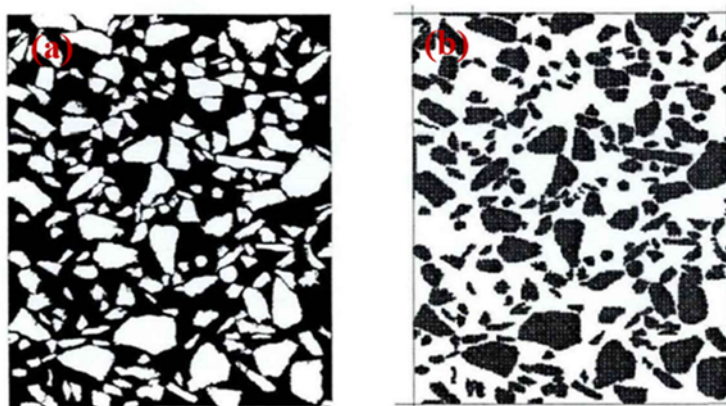
Figure 1. The application of image processing method in Particle Flow Code (PFC): (a) grayscale image of the specimen; (b) Discrete particle models.
