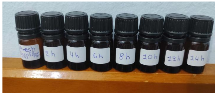
Figure 20. Sunflower oil samples. The labels indicate the total time inside the oven for each sample, at a temperature of 200 °C.
