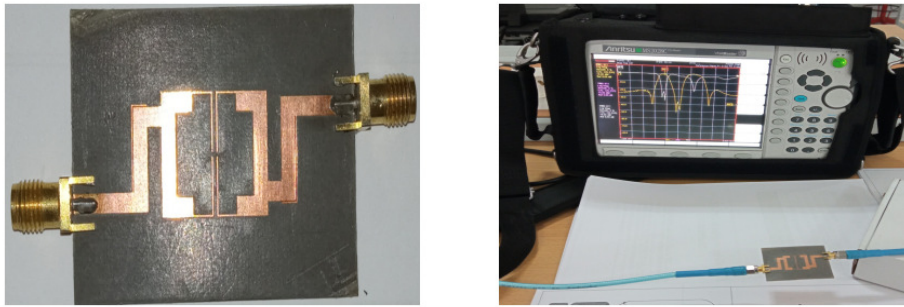
Figure 14. Photograph of the fabricated dual-band BPF with its measurement equipment.
