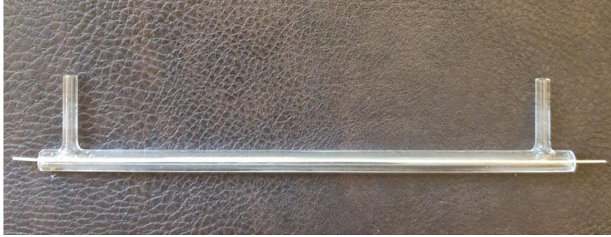
Figure 3. Reactor's glass body with an embedded silver-plated wire.
