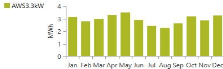
Figure 17. Monthly electricity production for system type 3B.
