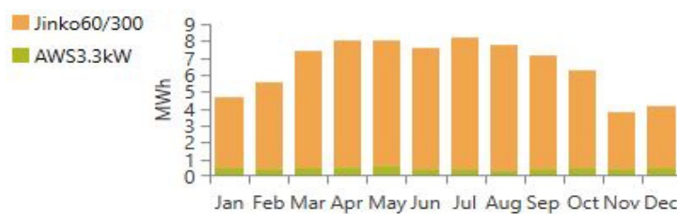
Figure 16. Monthly electricity production for system type 2B.
