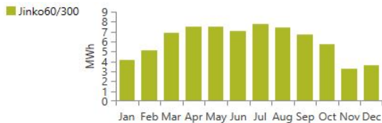
Figure 15. Monthly electricity production for system type 1B.
